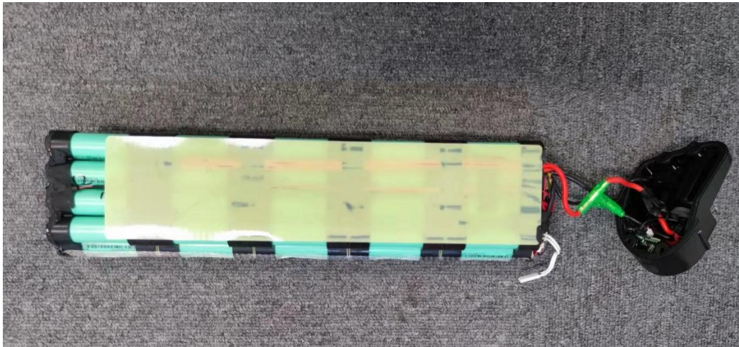
Figure 4 Internal view 2 of battery pack
