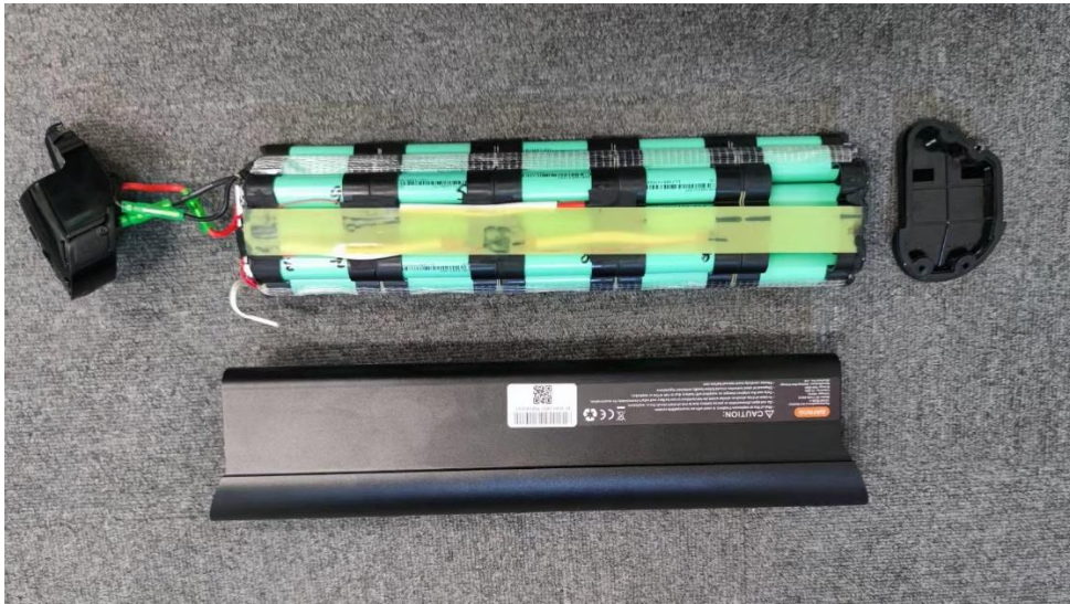
Figure 3 Internal view 1 of battery pack
